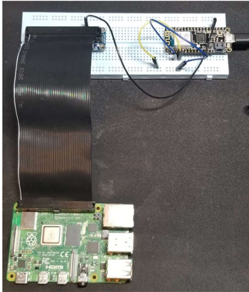
Figure 44: Early prototype to demonstrate communication over a faux Iridium SBD channel
