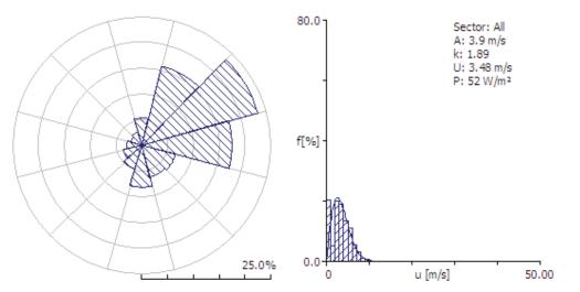
Figure 29: observed wind rose frequency diagram and the Weibull fit for JKIA\_Met' Station-Position: -1.32°N 36.92°E; Anemometer height: 10.00 m a.g.l. The WAsP prediction for the met. Station is given in the table below.
