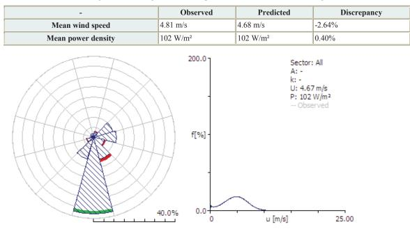
Figure 21: observed wind rose frequency diagram and the Weibull fit for Malindi\_Met' Station- Position: -3.23°N 40.10°E; Anemometer height: 10.00 m a.g.l. The WAsP prediction for the met. Station is given in the table below.
