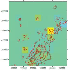
Figure 38: Modeled wind speeds at 50m a.g.l. a.g.l.
