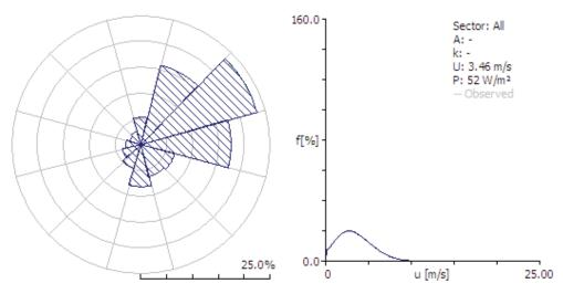
Figure 30: The WAsP predicted wind rose frequency diagram and the Weibull fit for JKIA\_Met' Station- Position: -1.32°N 36.92°E; Anemometer height: 10.00 m a.g.l.
