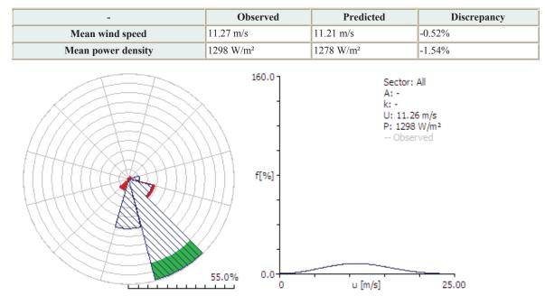
Figure 37: The WAsP predicted wind rose frequency diagram and the Weibull fit for Marsabit\_Met' Station-Position: 2.32°N 37.98°E; Anemometer height: 10.00 m a.g.l.
