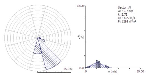
Figure 36: The observed wind rose frequency diagram and the Weibull fit for Marsabit Met -Position: 2.32°N 37.98°E; Anemometer height: 10.00 m a.g.l.
