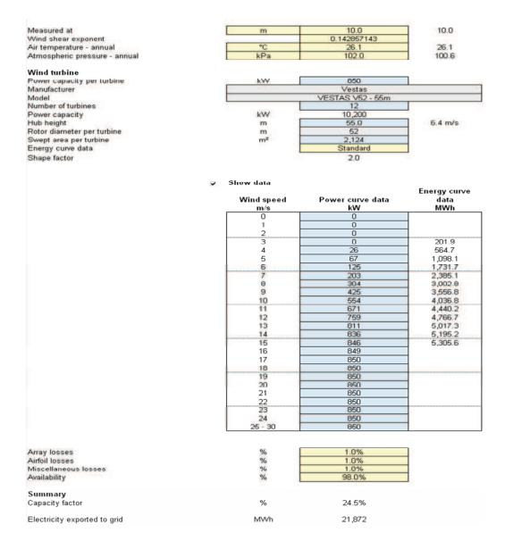
From the table above a summary of the wind resource and the turbine conversion shows that at Ras Ngomeni a turbine will yield gross production of 1917 MWh at a specific yield of 858 kWh per square meter. The wind available provide a capacity factor of 24.5% considered a conservative assessment compared with the operational history of the two turbine farm on Ng'ong Hills near Nairobi.
